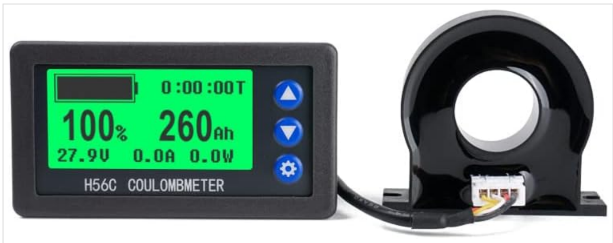
Image 1: Taidacent H56CH Digital Hall Coulomb Counting Battery Monitor and its accompanying current sensor (shunt). The monitor displays battery percentage, capacity, voltage, current, and power. The shunt is connected via a cable to the monitor.
