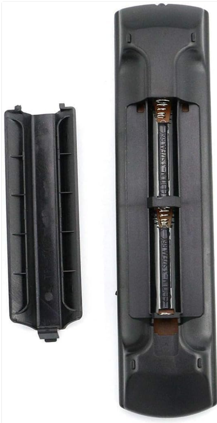
Image: Back of the remote control with the battery cover removed, revealing the two AAA battery slots.
