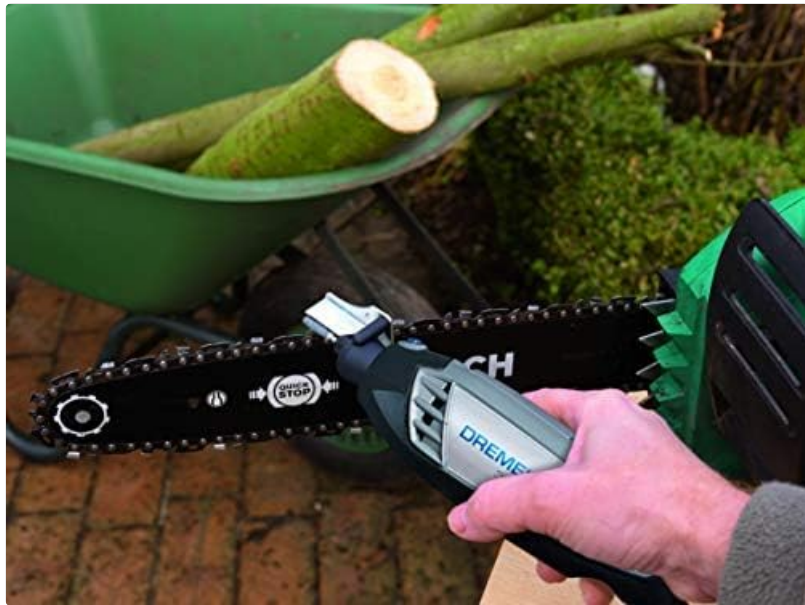
Figure 2: The Dremel rotary tool with the sharpening attachment correctly installed and positioned on a chainsaw chain, ready for sharpening.
