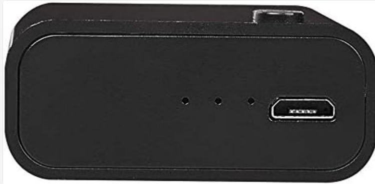
Image: A close-up side view of the Jensen RBTTX10, showing the micro-USB charging port and three small indicator lights. Familiarize yourself with the device's ports and controls:
