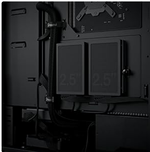
Figure 4: SSD mounting locations behind the motherboard tray.
