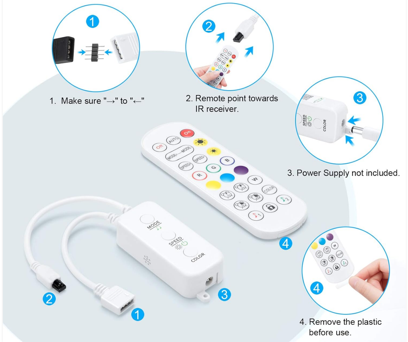
Figure 4: Connection and usage tips for the LED strip controller.
