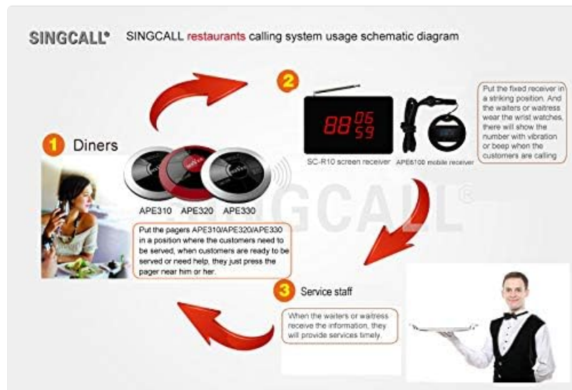
Figure 2.1: Schematic diagram illustrating the usage of the SINGCALL restaurant calling system. It shows diners pressing pagers, which send signals to a screen receiver and a mobile receiver worn by service staff, enabling efficient service.
