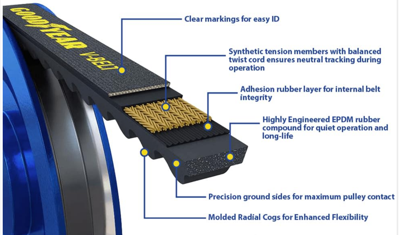
Image: Cross-section diagram illustrating the internal components of a Goodyear V-Belt, including clear markings for identification, synthetic tension members, adhesion rubber layer, EPDM rubber compound, precision ground sides, and molded radial cogs for enhanced flexibility.
