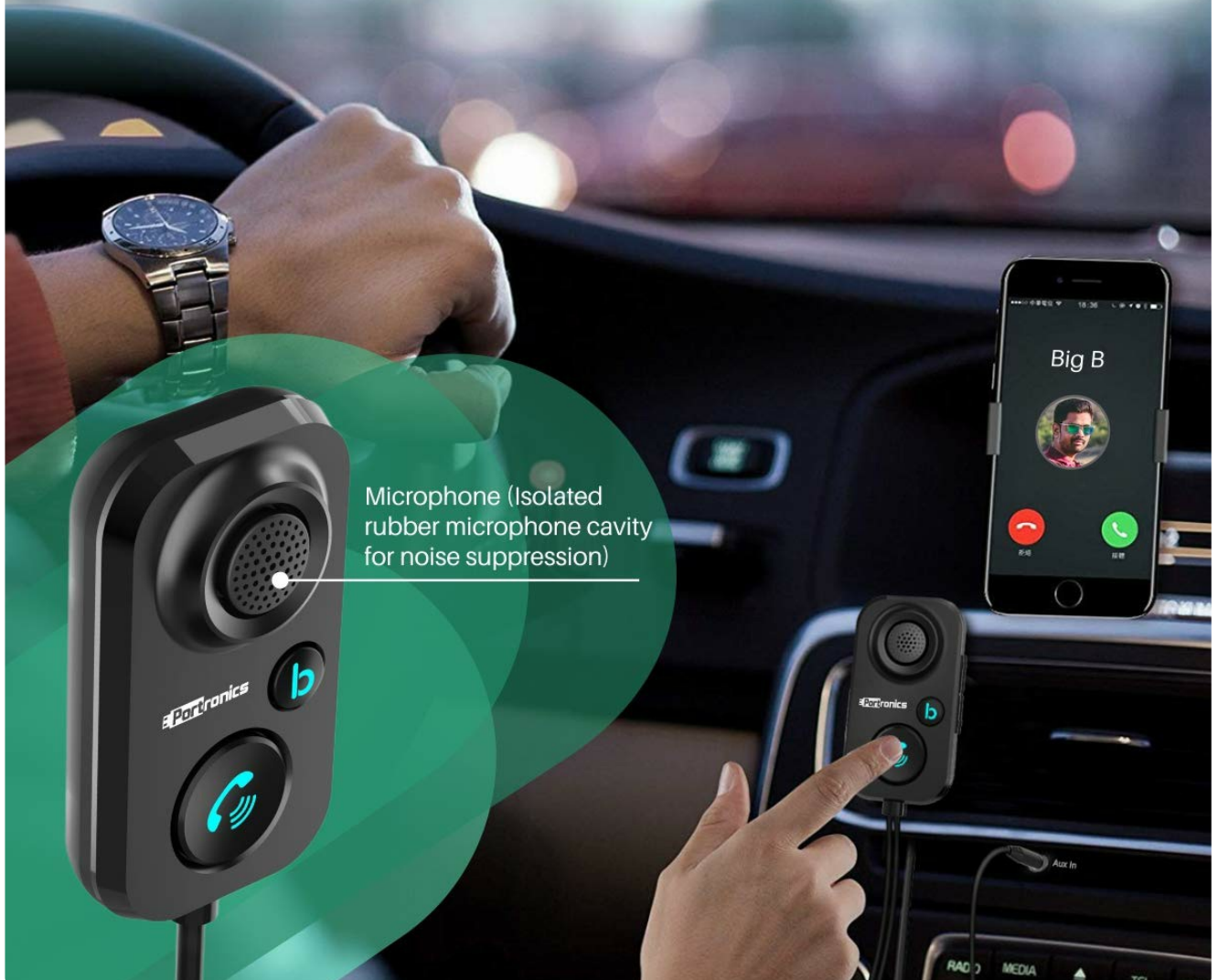
Figure 6: The Portronics AUTO 12 in use for hands-free calling, showing the microphone and call button, with a phone displaying an incoming call.
