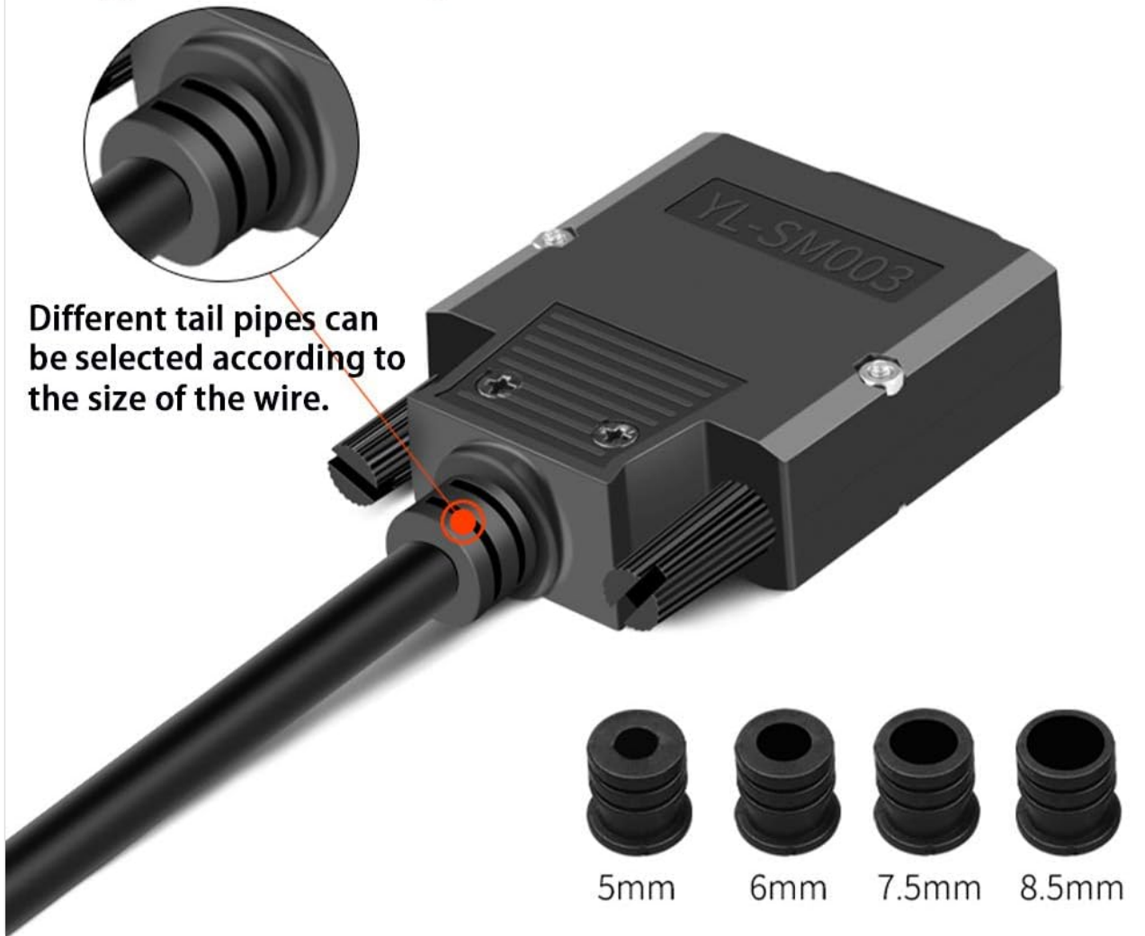
Image 5.1: An image showing the various tail pipe sizes (5mm, 6mm, 7.5mm, 8.5mm) and how they are used to secure the cable at the connector's entry point, preventing strain.
