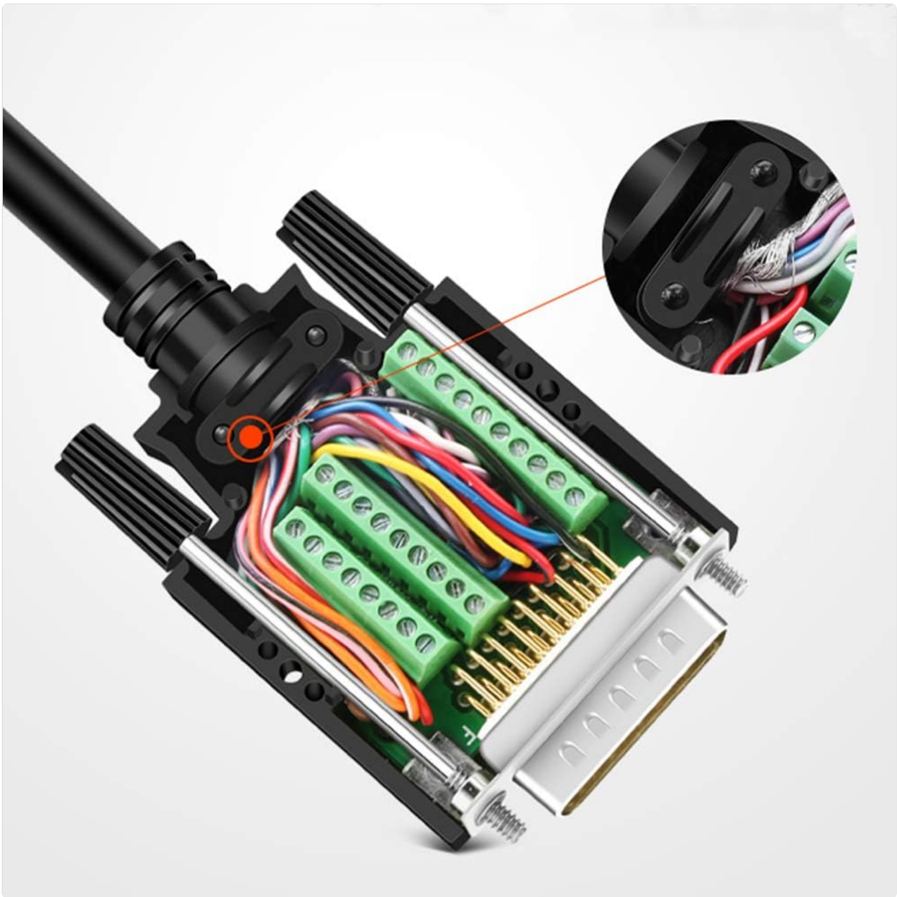
Image 5.3: An internal view of the connector showing multiple colored wires connected to the terminal block, demonstrating a typical wiring configuration.
