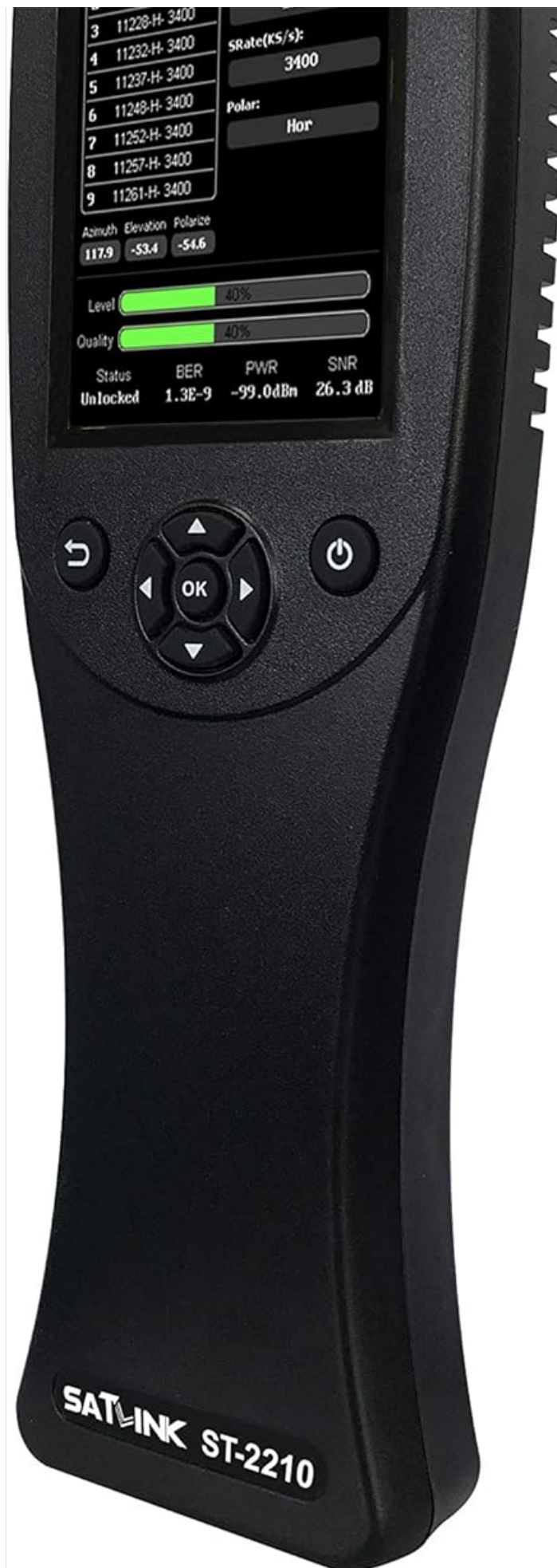
Figure 6: The ST-2210 display showing real-time signal parameters, including Level, Quality, BER, PWR, and SNR, essential for satellite dish alignment.
