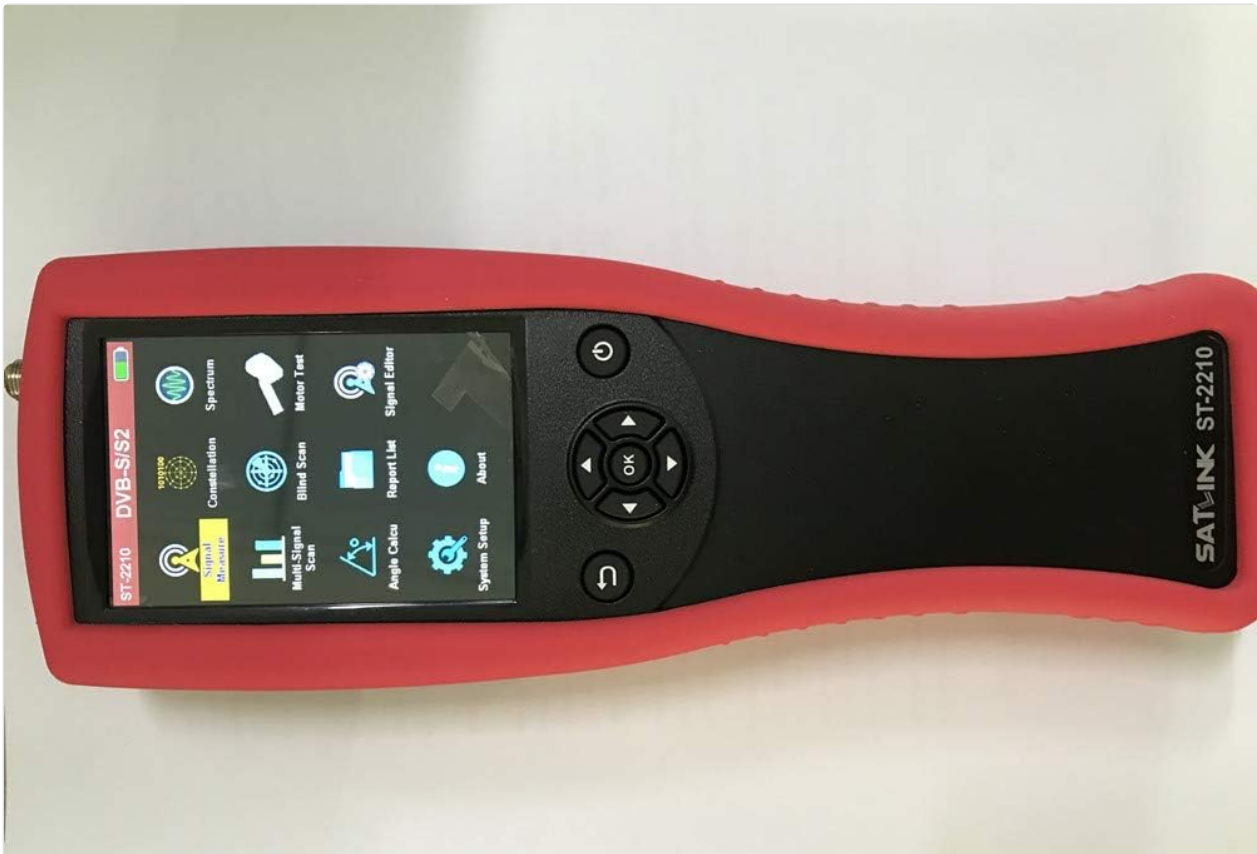
Figure 5: The main menu interface of the ST-2210, showing various functions such as Signal Monitor, Constellation, Spectrum, and System Setup.
