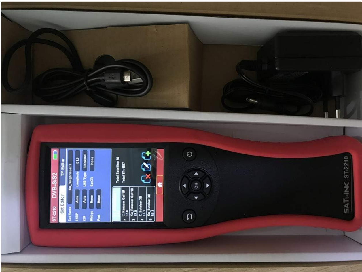
Figure 2: The SATLINK ST-2210 device along with its accessories, including the silicone case, USB upgrade cable, and AC adapter.
