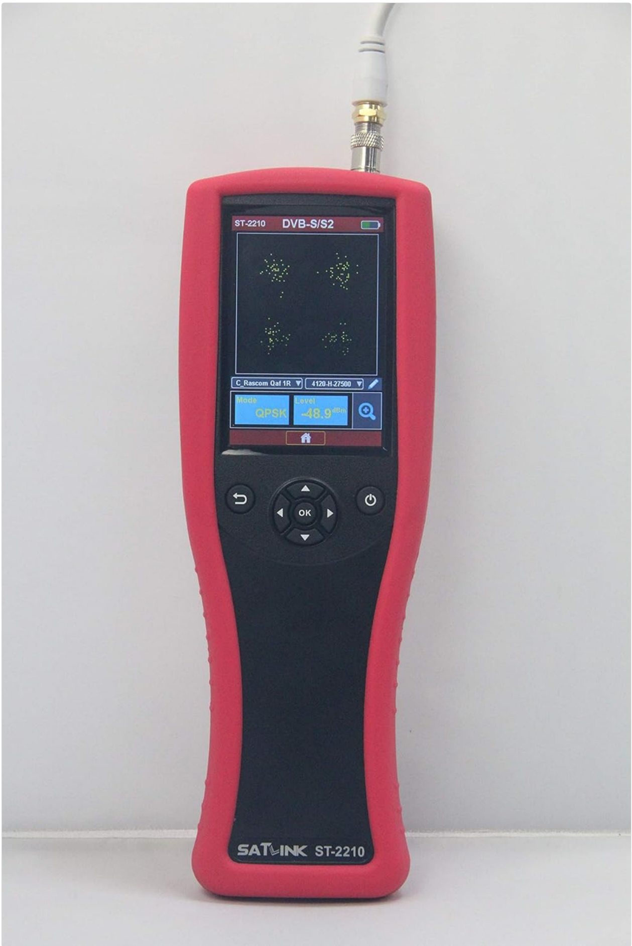
Figure 4: The ST-2210 in its protective silicone case, connected to a satellite coaxial cable for signal reception.
