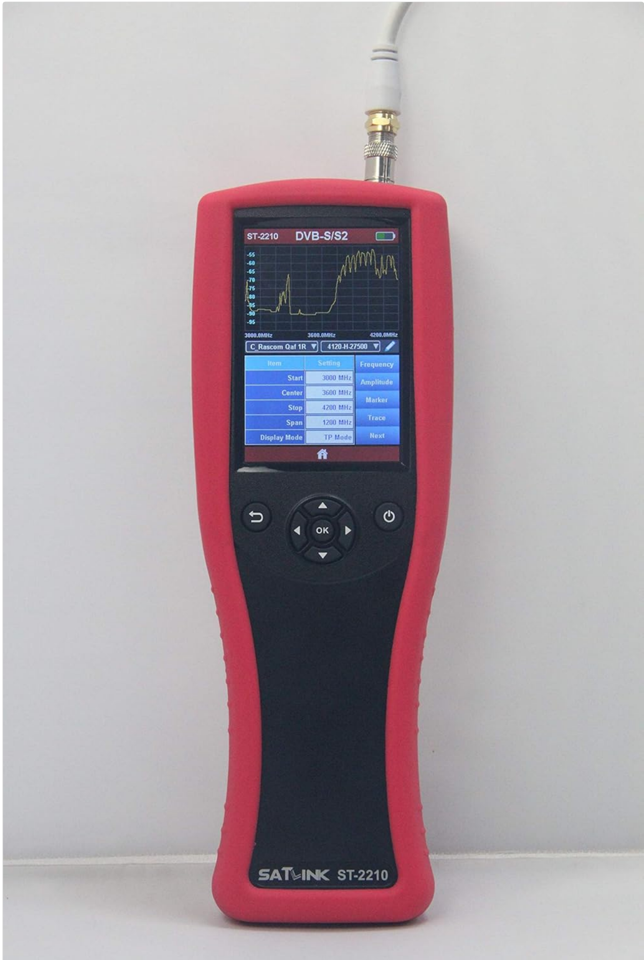
Figure 8: The ST-2210 screen showing the spectrum analyzer, which graphically represents signal strength across different
