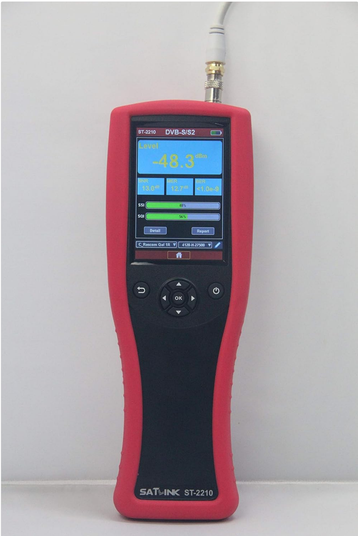
Figure 7: The ST-2210 displaying a prominent signal level reading in dBm, indicating the strength of the received satellite signal.
