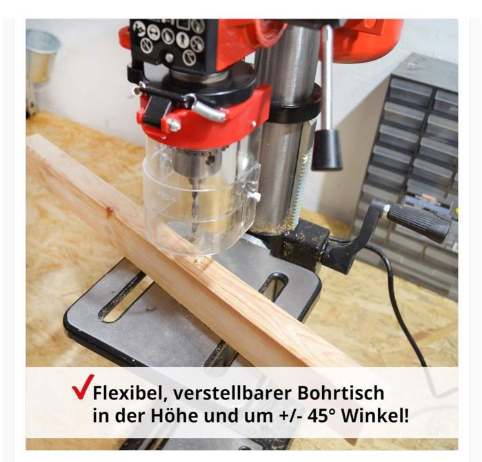
The pillar drill in use, demonstrating the adjustable drilling table set at an angle for precise material positioning.
