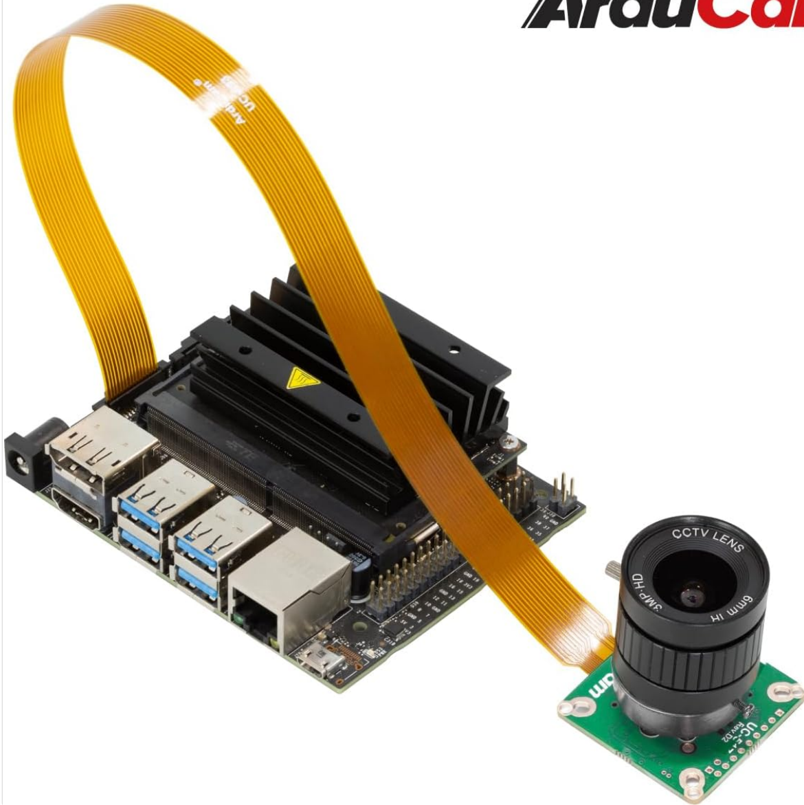
Figure 5: The Arducam IMX477 HQ Camera Board connected to a Jetson Developer Kit using the flexible flat cable.
