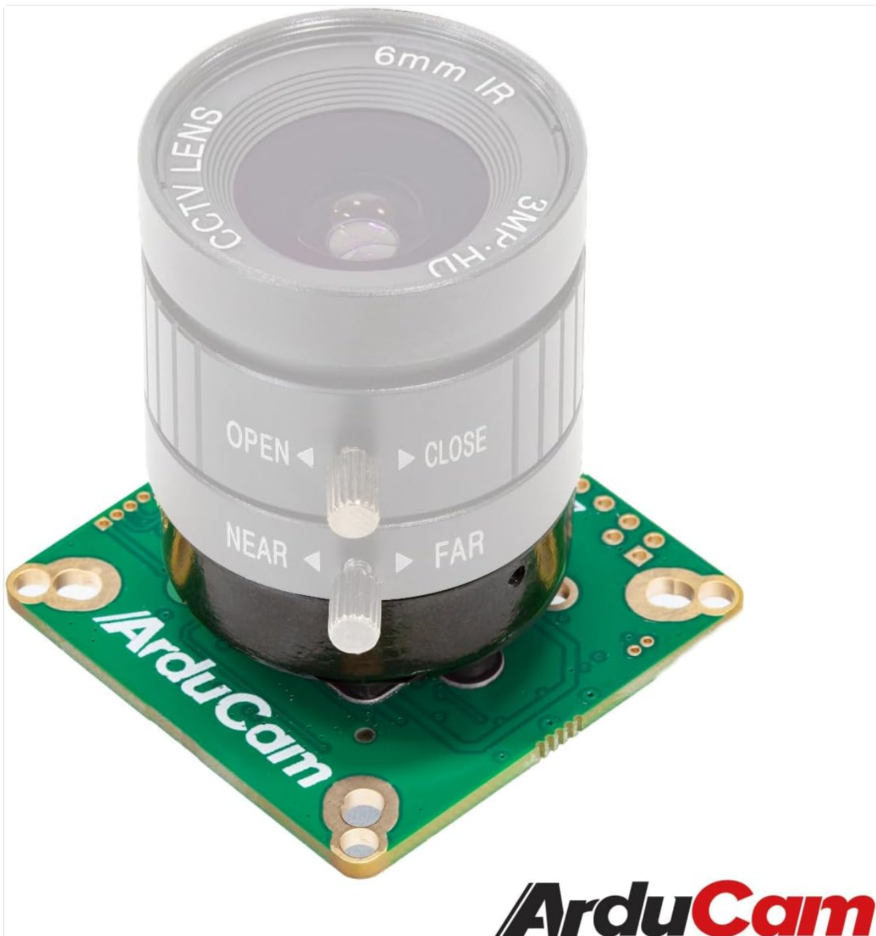
Figure 4: The Arducam IMX477 HQ Camera Board with a 6mm IR CCTV lens securely attached to the CS-mount.
