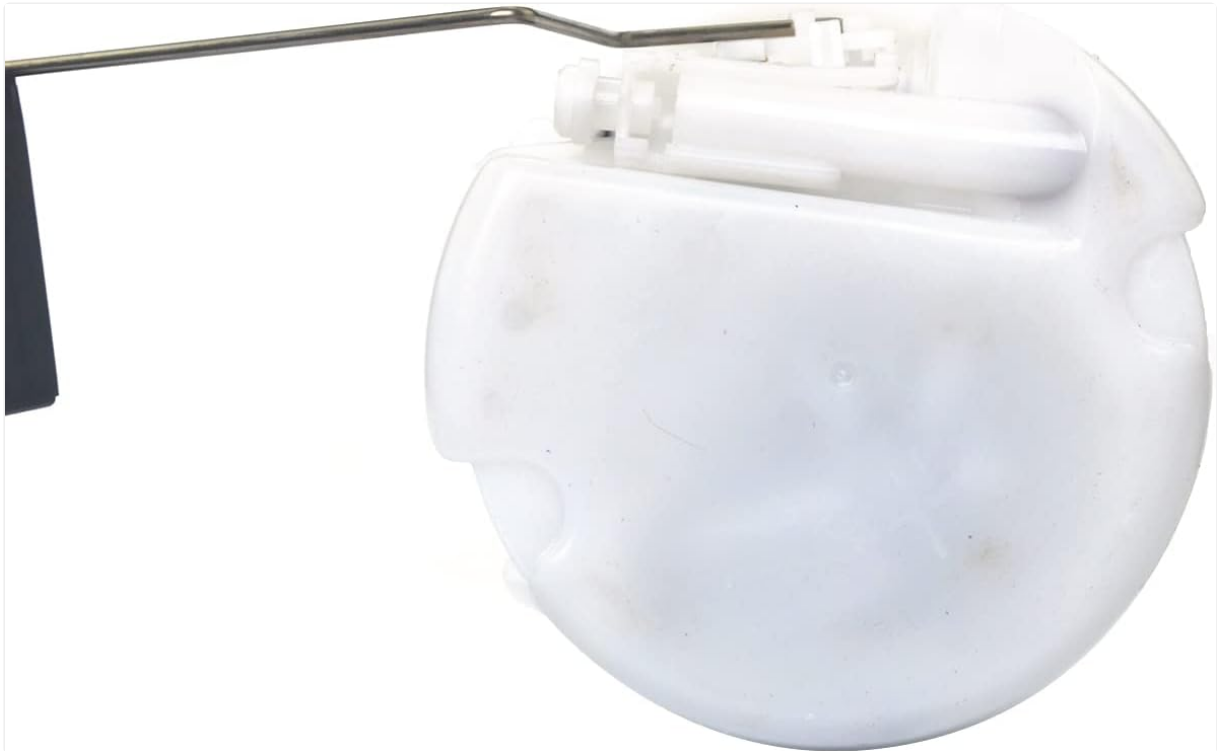
Figure 3.5: Bottom view of the fuel pump module, illustrating the fuel level float mechanism.
