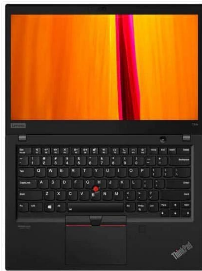
Figure 3.2.1: A top-down view of the Lenovo ThinkPad T14s Gen 1 keyboard, highlighting the red TrackPoint in the center of the keyboard and the associated mouse buttons below the spacebar. This image demonstrates the primary input devices for navigation and typing.
