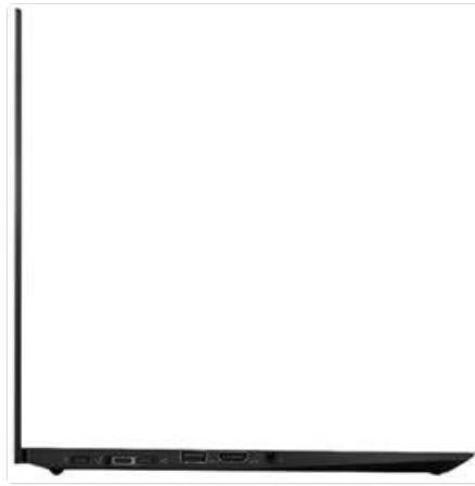
Figure 3.4.1: The left side of the Lenovo ThinkPad T14s Gen 1, displaying its various ports including USB-C (Thunderbolt 3), USB-C (Power Delivery), USB 3.2 Gen 1, HDMI, and a headphone/microphone combo jack. This view highlights the connectivity options available on this side of the laptop.
