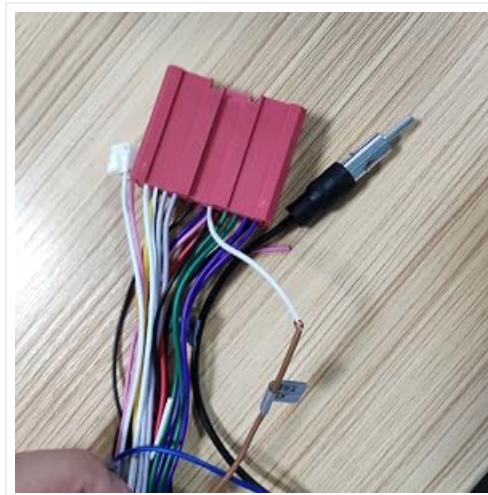
Figure 2.3: Wiring modification for steering wheel control. The 6th pin beside the black cable (counting from the right) may need to be cut and connected to the 'Key 1' wire.
