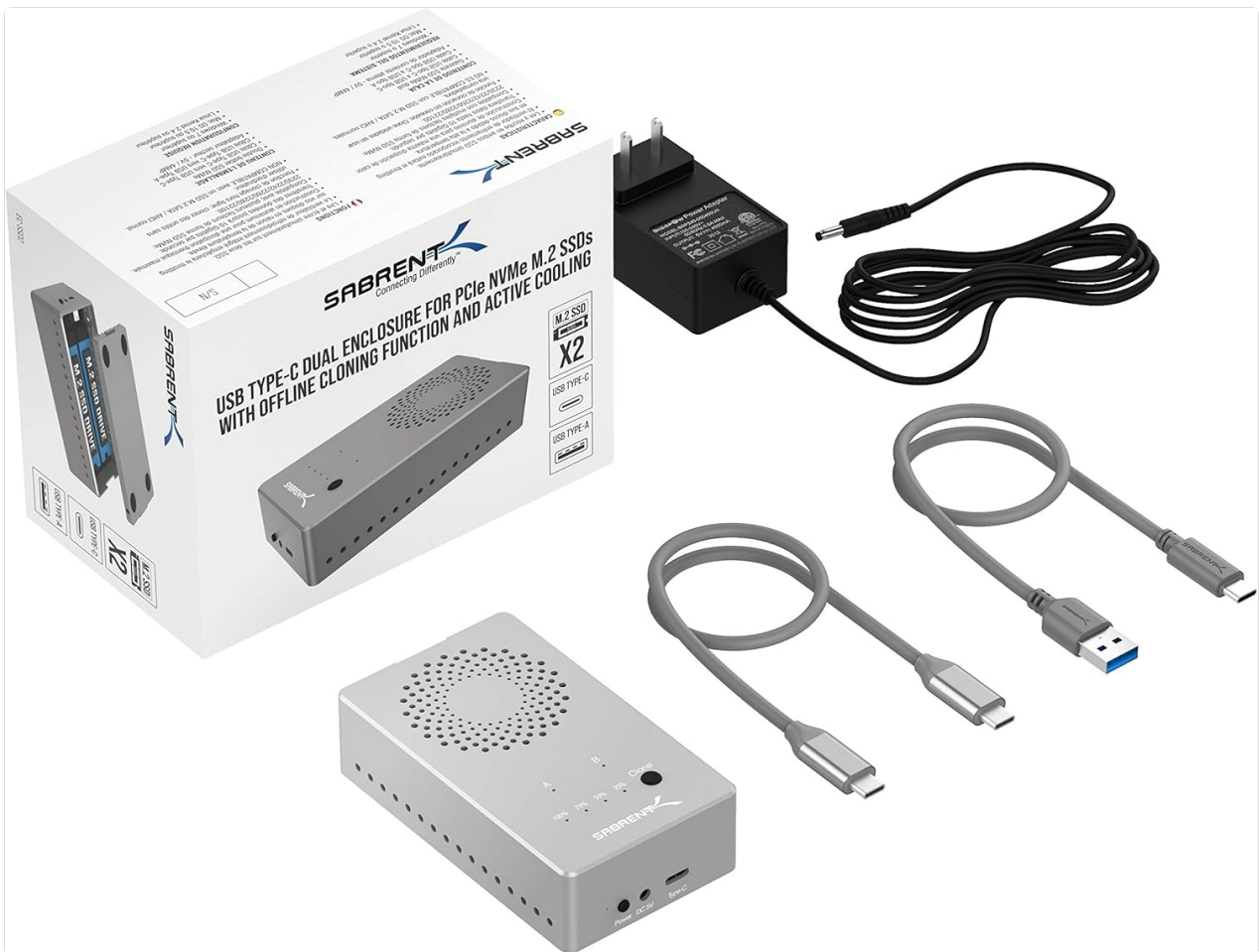
Image 2.1: Contents of the SABRENT EC-SSD2 package, including the docking station, cables, and power adapter.
