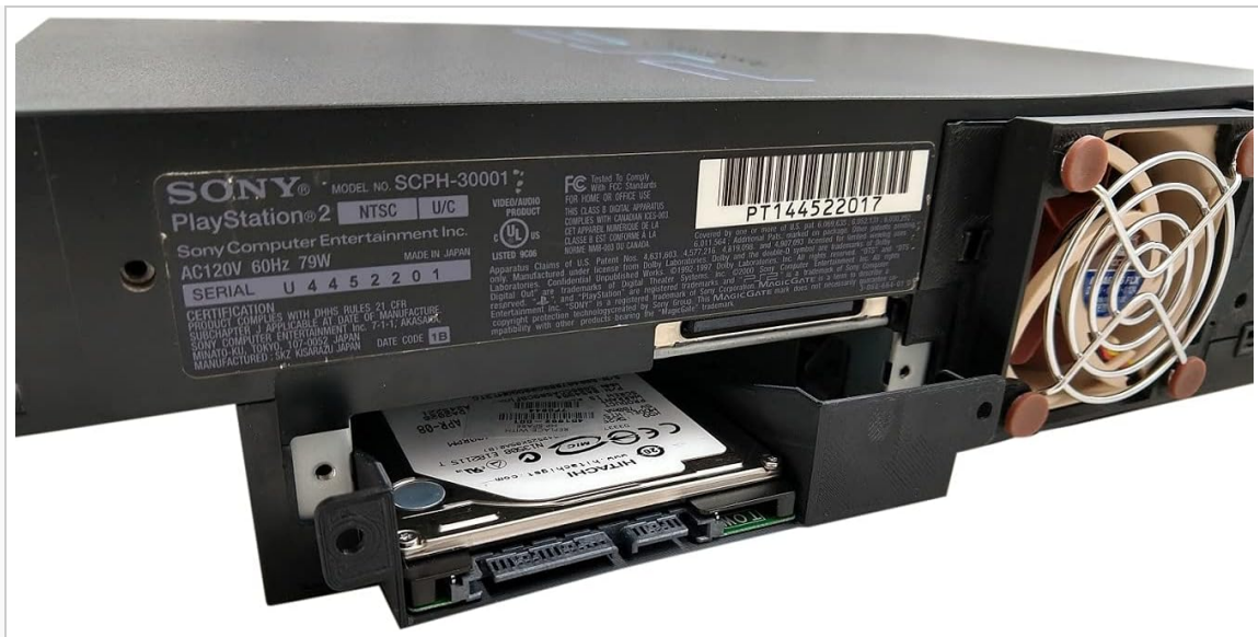
Image 3: The REUUY spacer with an installed 2.5-inch drive, positioned within the expansion bay of a PlayStation 2 Fat console. This view shows the rear of the console with the drive assembly inserted.
