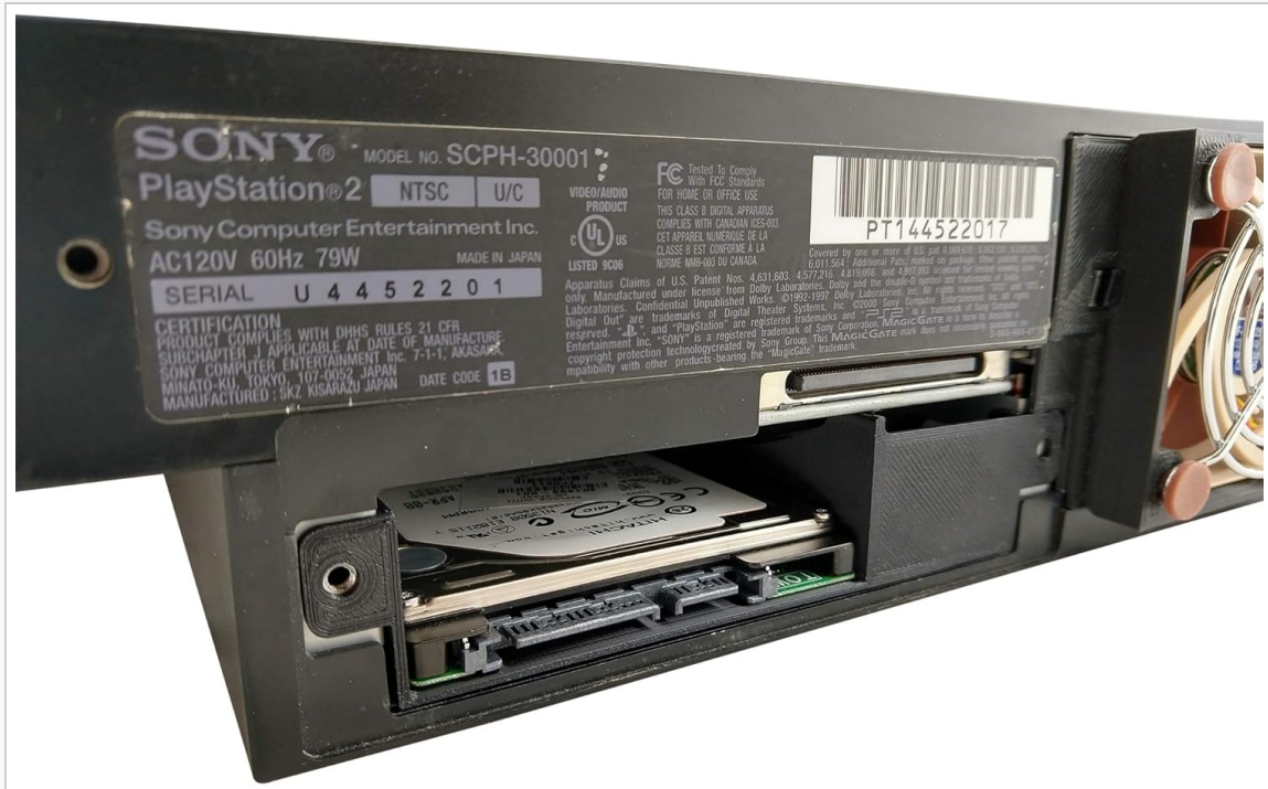
Image 4: A PlayStation 2 Fat console (model SCPH-30001) with the REUUY spacer and 2.5-inch drive fully installed in the rear expansion bay. The console's serial number and model details are visible.
