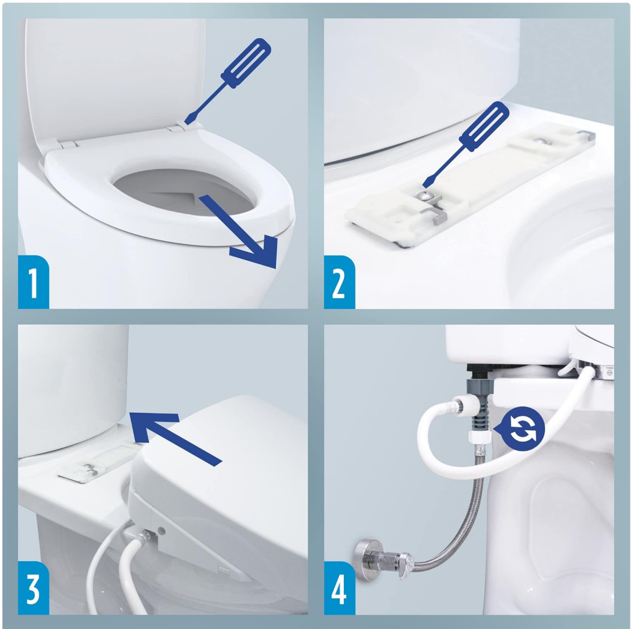
This image provides a visual overview of the installation process: 1. Remove existing toilet seat. 2. Install mounting bracket. 3. Slide WASHLET onto bracket. 4. Connect water supply and power.
