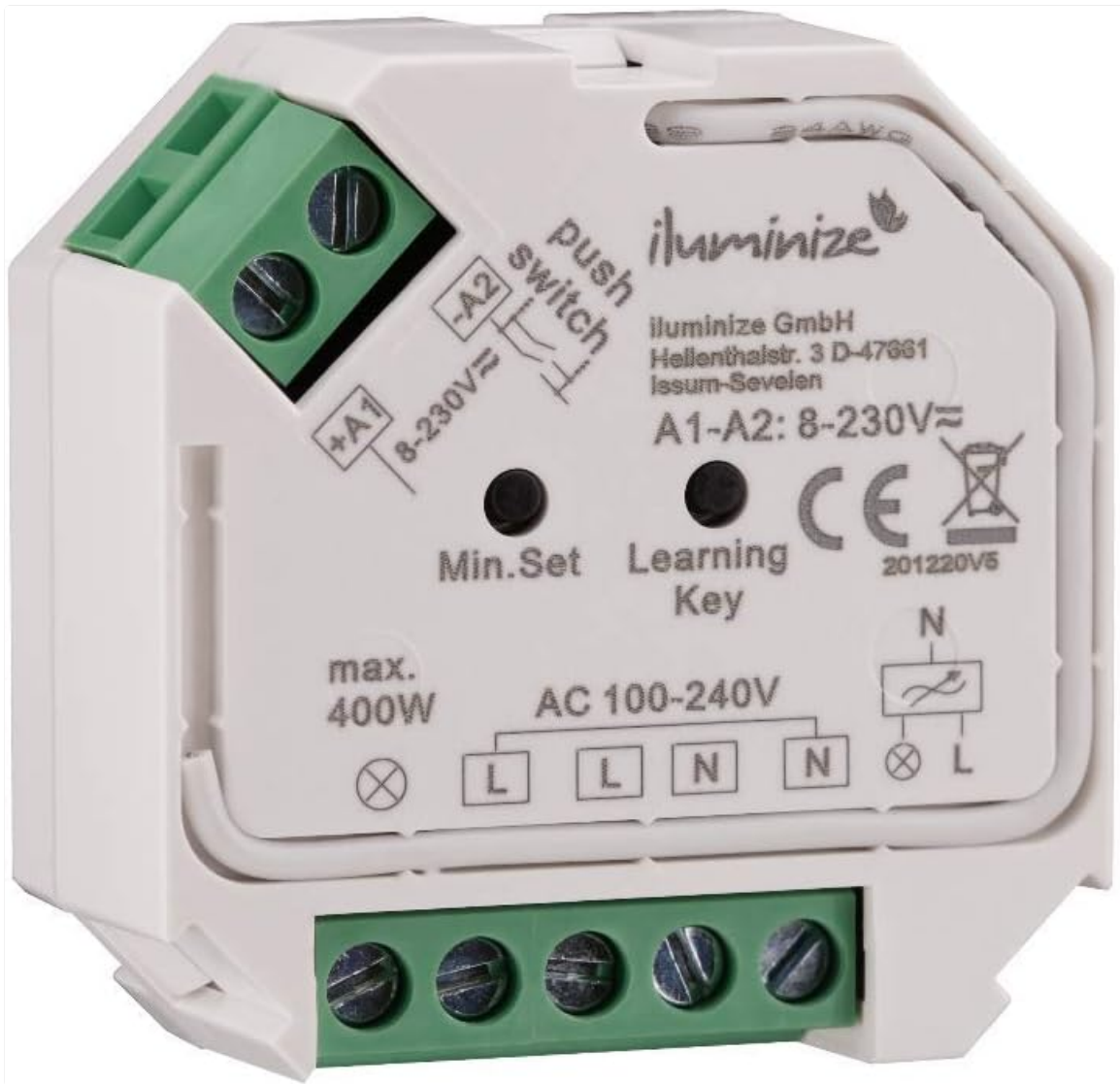
Front view of the iluminize Dimm-Aktor 500.201, showing connection terminals for L (Live), N (Neutral), and output to the lamp, along with 'Min.Set' and 'Learning Key' buttons. Input voltage range is AC 100-240V, max 400W.
