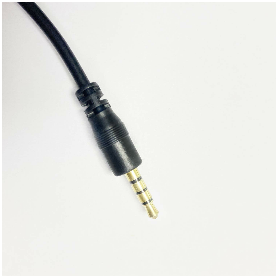
Image: Close-up of the 3.5mm jack connector on the sensor probe cable, ready for connection to the controller.
