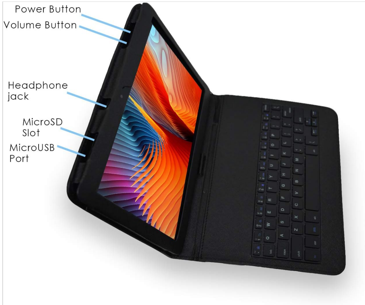
Image showing the Azpen A1080 tablet securely placed within the keyboard case, highlighting the accessible power button, volume button, headphone jack, MicroSD slot, and Micro USB port on the tablet's side.
