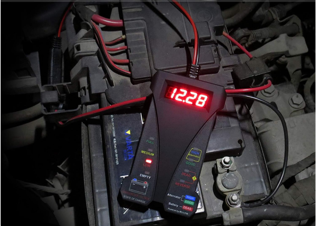
Figure 6.2: MP0514A Battery Tester in use within a vehicle's engine bay.
