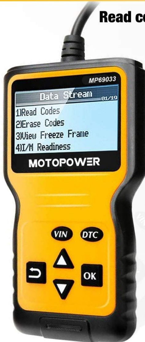
Figure 6.7: MP69033 OBD2 Code Reader showing various diagnostic screens.
