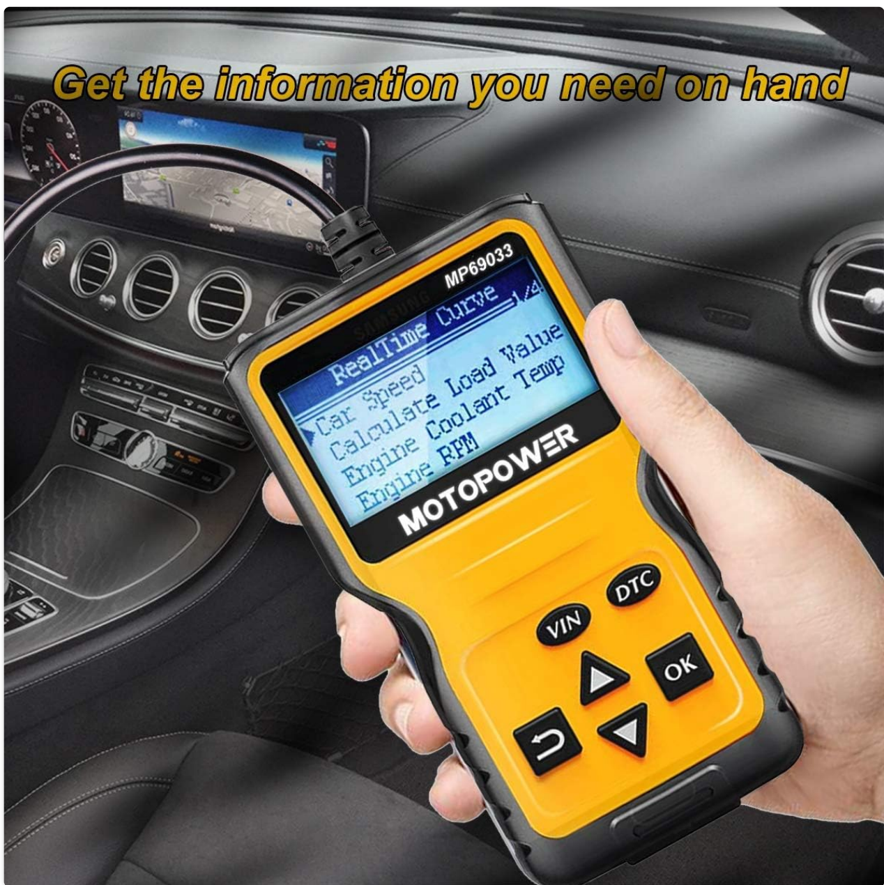
Figure 6.8: MP69033 OBD2 Code Reader displaying real-time data in a vehicle.
