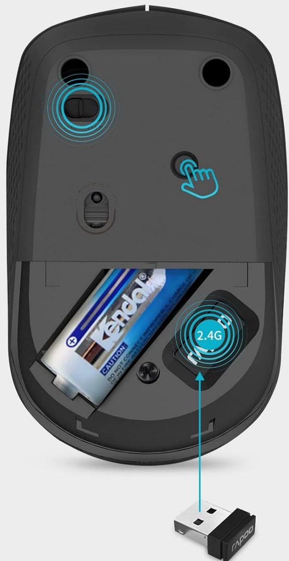
Figure 3: Underside of the mouse showing the battery compartment, USB receiver storage, and connection buttons.
