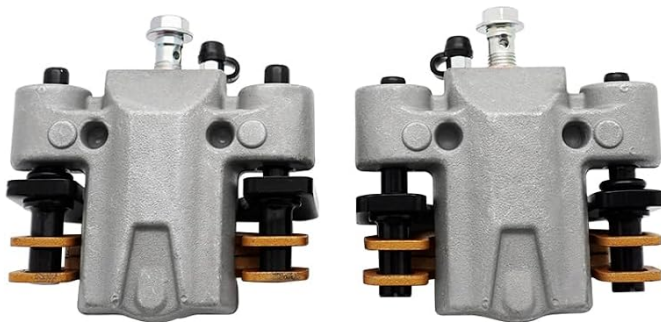
Figure 5: Caliper features: Mounting bracket and brake pads.
