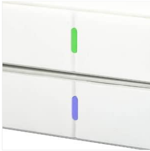
Image: The LED indicator on the WSA-5TR-V2 unit, which changes color to signify the active frequency band (blue for 5.8GHz, green for 5.2GHz).
