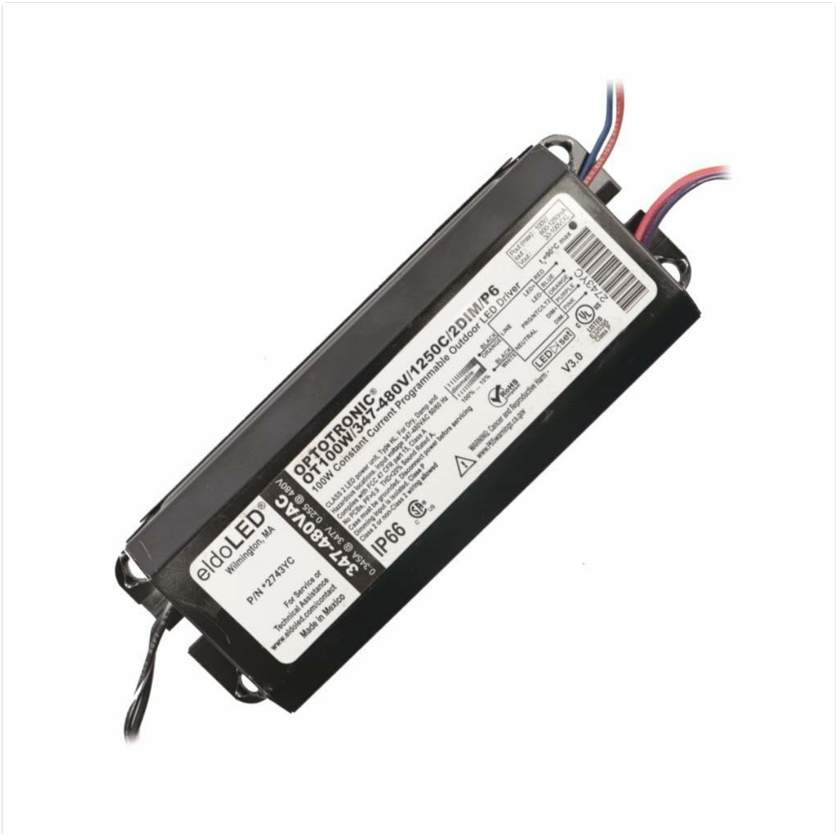
Figure 1: Osram OT100W/347-480V/1250C/2DIM/P6 LED Power Supply. The label on the device details its model number, input voltage (347-480VAC), output current range (600-1250mA), dimming capabilities, and wiring connections for line, neutral, LED output, and dimming control.
