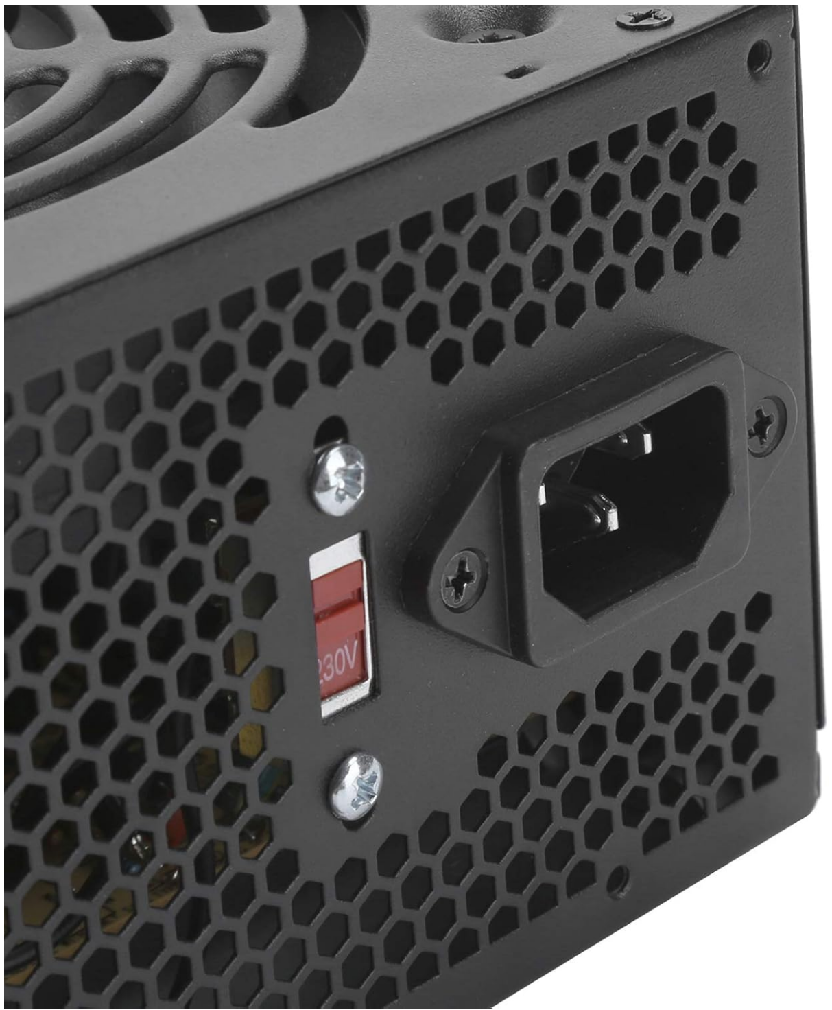
Figure 5.1: The voltage selector switch and AC power input on the rear of the power supply. Ensure the switch is set to the correct local voltage (115V or 230V) before connecting to power.
