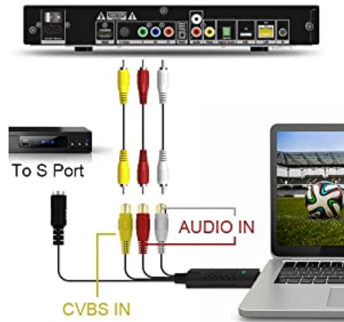
Image: A diagram illustrating how to connect a video source (like a DVD player) to a laptop using the VIXLW capture card, showing both CVBS (RCA) and S-Video input options.
