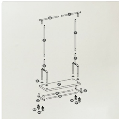
Image 3.1: Exploded diagram showing all individual parts of the garment rack, including pipes, connectors, the wooden base, and wheels, along with labeled hardware.
