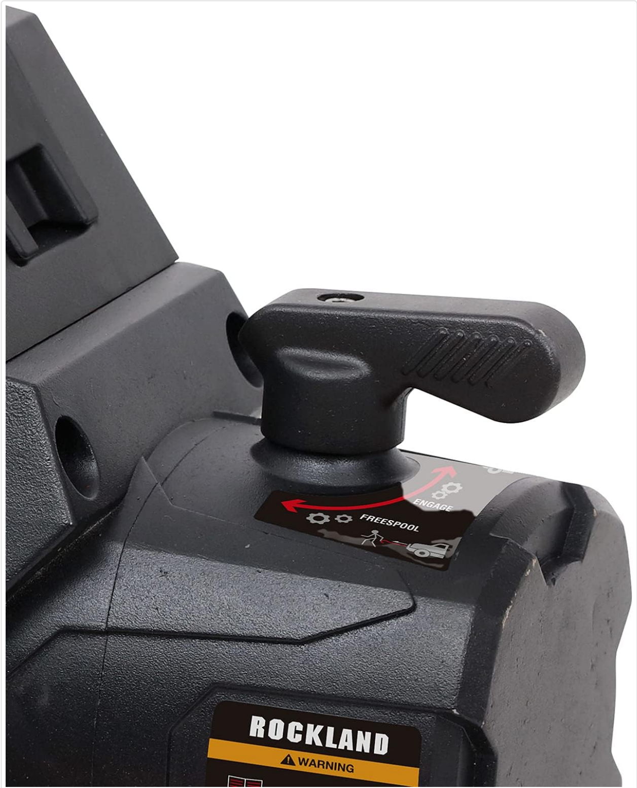
Figure 4.1: The clutch lever, used to switch between free spooling and engaged winching modes.
