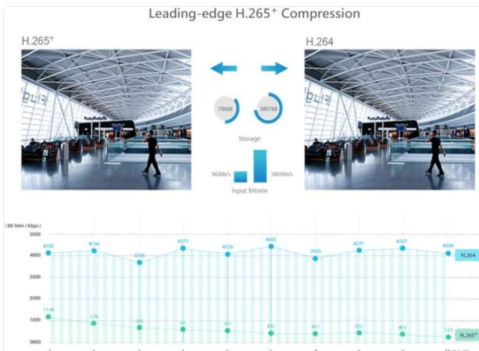
Figure 3: Illustration demonstrating the superior compression efficiency of H.265+ compared to
