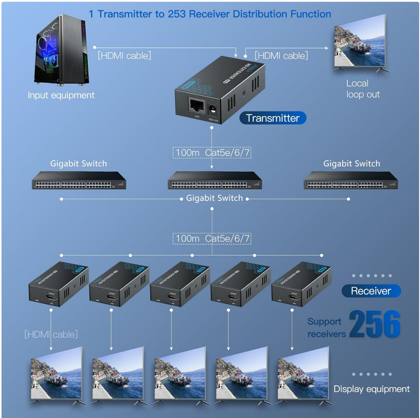
This diagram illustrates an advanced setup for the PWAY HDMI Extender, where a single Transmitter unit distributes the HDMI signal across multiple interconnected Gigabit Ethernet Switches. This allows for signal extension and distribution to numerous Receiver units and displays over a larger, more complex network infrastructure.
