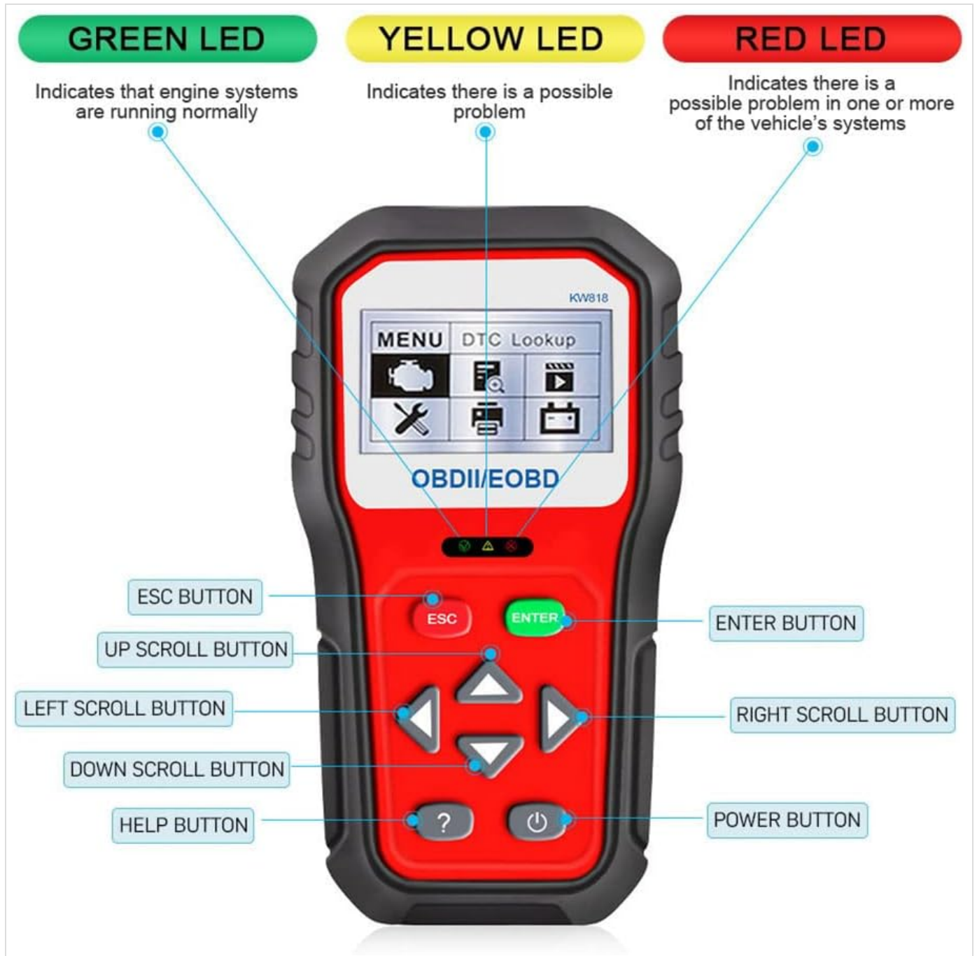
Diagram illustrating the scanner's button layout (ESC, ENTER, Up, Down, Left, Right, Help, Power) and the meaning of the Green, Yellow, and Red LED indicators for system status.
