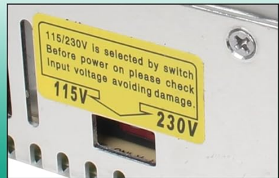
Image: Terminals and voltage selection switch on the 350W 24V DC Switching Power Supply.
