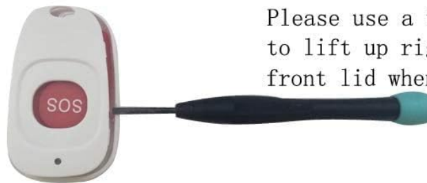
Image 4.1: Visual guide for plugging in the receiver and wearing the SOS button. Also demonstrates the method for opening the transmitter to replace the battery.
