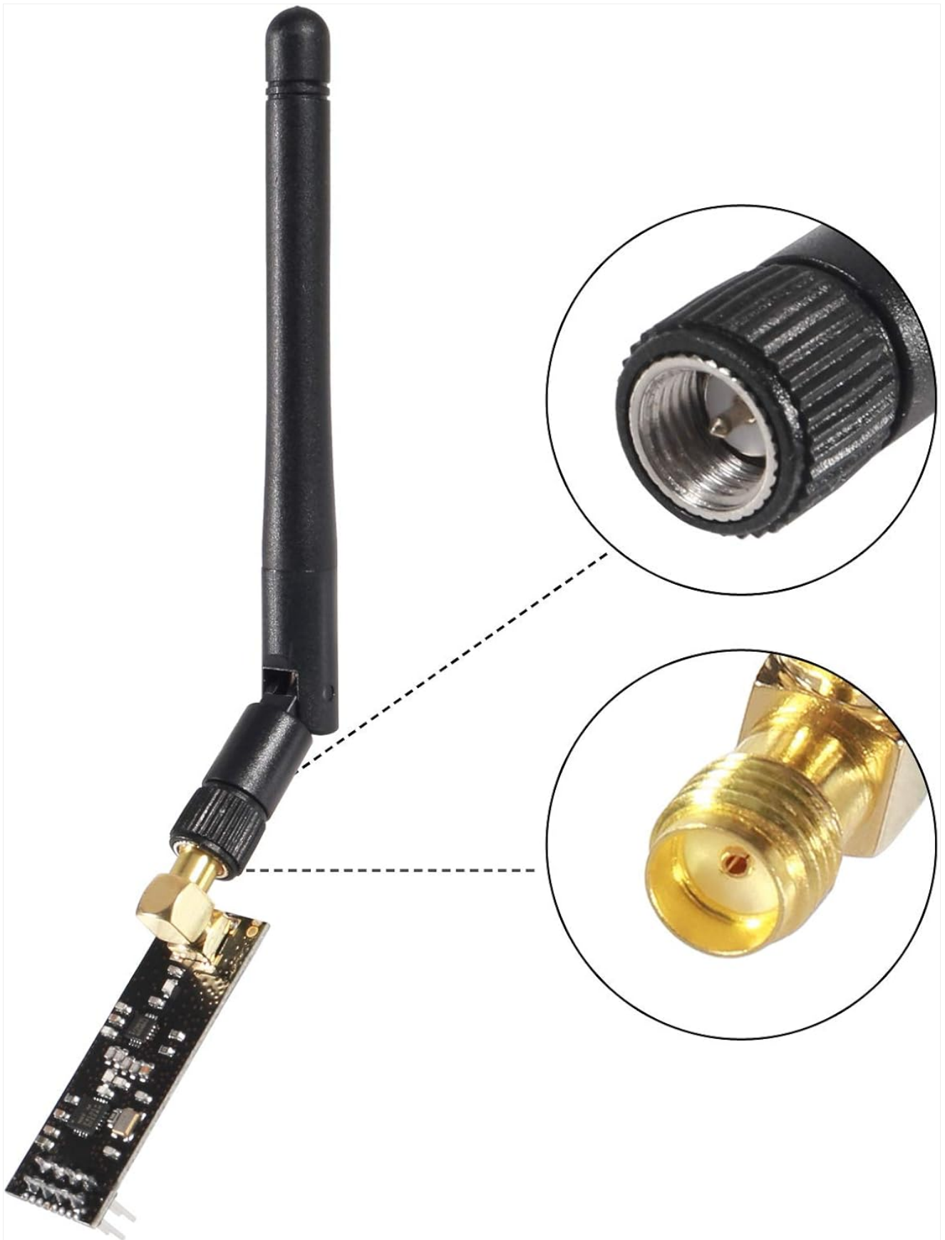
Figure 5: Illustration of how to connect the SMA antenna to the NRF24L01+PA+LNA module.
