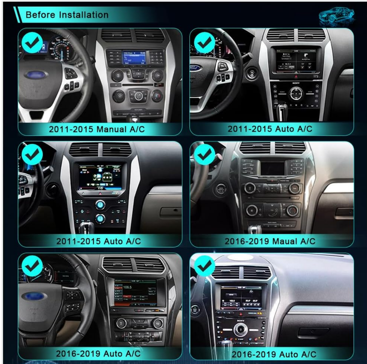
Figure 4.1: Dashboard configurations for Ford Explorer 2011-2019, showing differences between Manual A/C and Auto A/C systems across different model years. This helps identify your vehicle's specific setup before installation.
