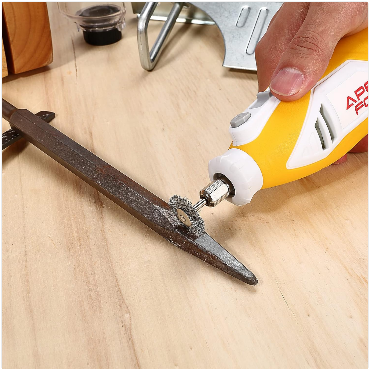
Figure 6.3: A wire brush accessory effectively cleans and prepares metal surfaces.
