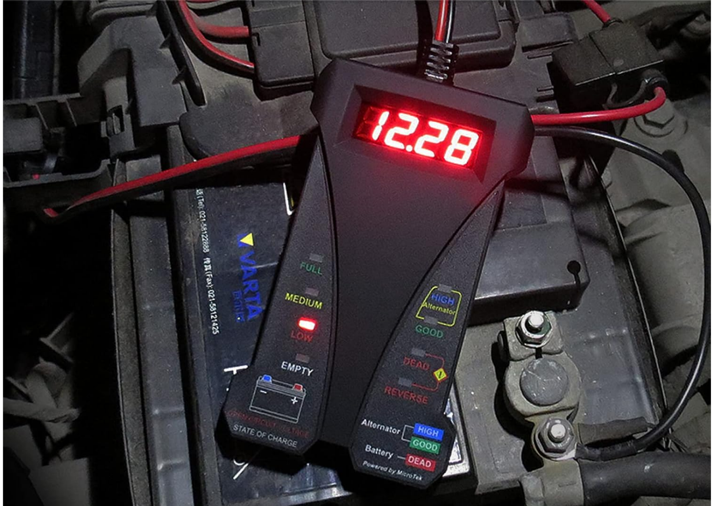
Image: MOTOPOWER MP0514A Battery Tester connected to a car battery, displaying voltage and indicating alternator/charging system status.
