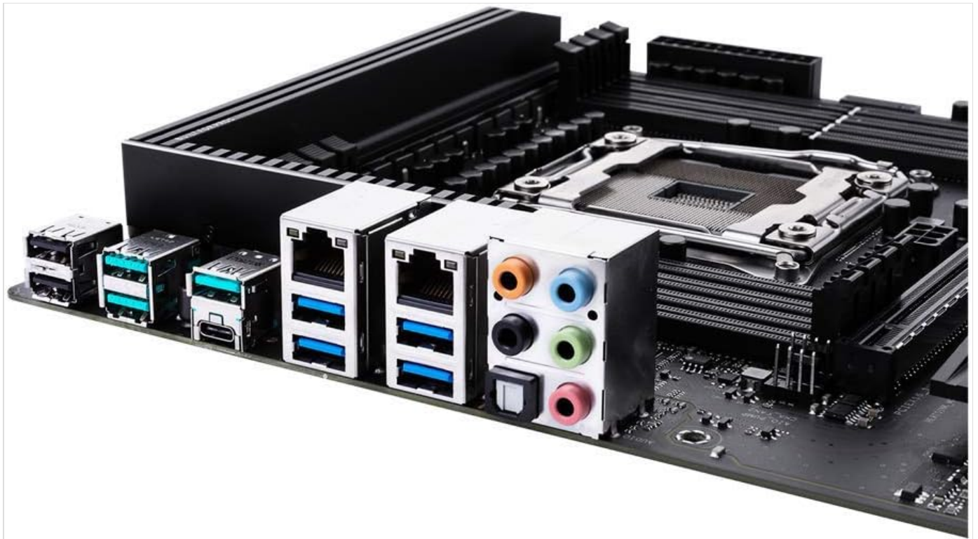
Figure 2.2: An angled view of the ASUS Pro WS C422-ACE motherboard, showing the rear I/O panel with various ports for external connections.
