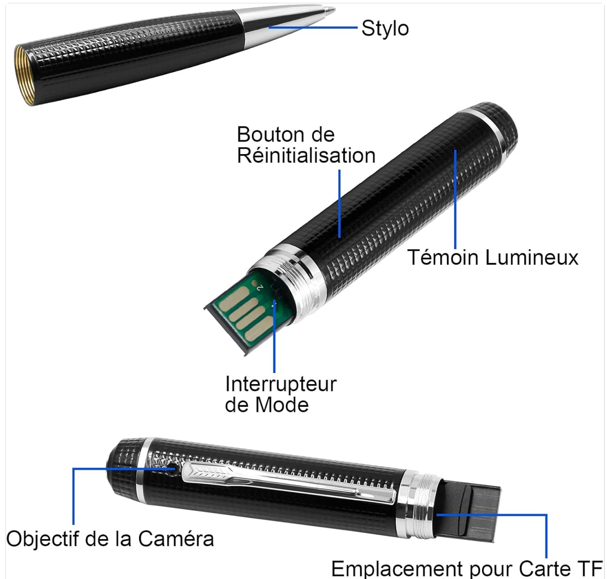
Image: Labeled diagram of the spy camera pen, indicating the pen tip, reset button, indicator light, mode switch, camera lens, and TF card slot.
