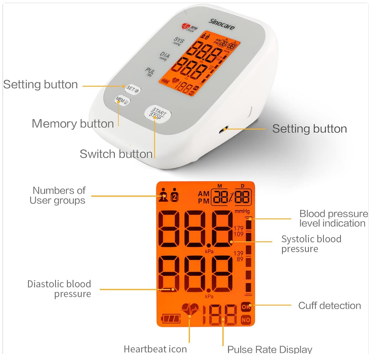
Image 4.2: An annotated image highlighting the display elements and buttons: Setting button, Memory button, Start/Stop button, User group indicator, Blood pressure level indication, Systolic and Diastolic pressure, Pulse Rate, Heartbeat icon, and Cuff detection indicator.
