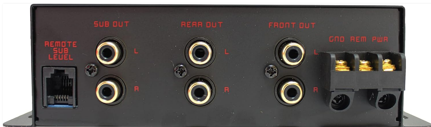
Image: Subwoofer, Rear, and Front RCA output connections, along with the remote bass level port and power terminals (GND, REM, PWR) on the American Bass ABX 3.1A electronic crossover.
