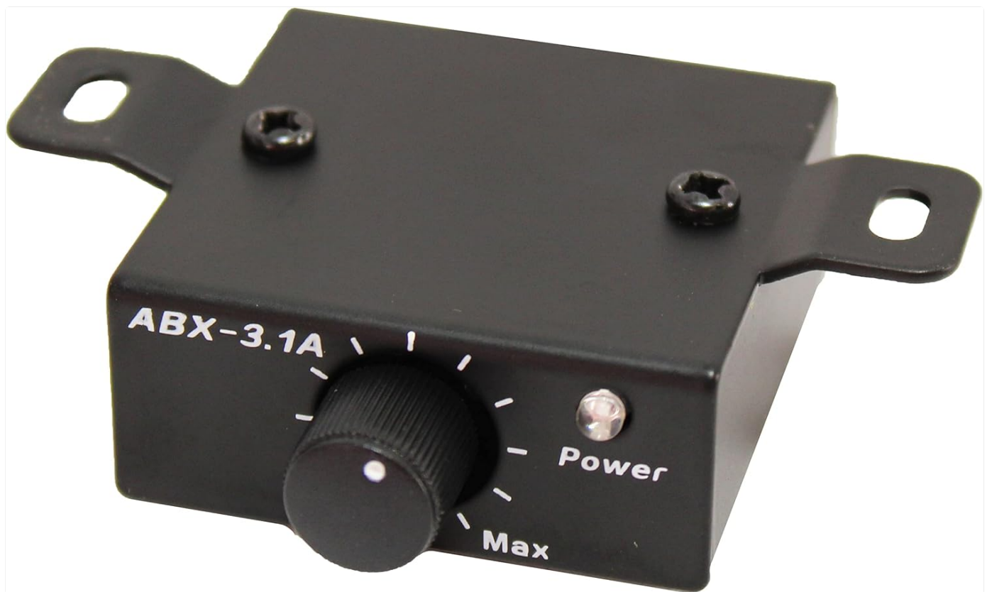
Image: The remote bass knob for the American Bass ABX 3.1A, featuring a rotary control for bass level adjustment and a power indicator LED.
