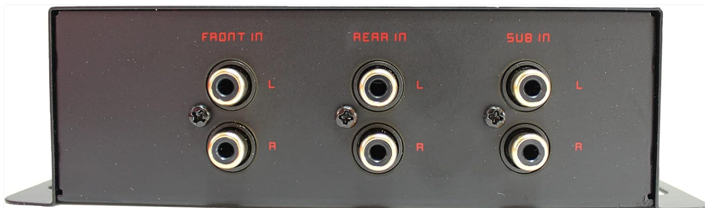
Image: Front, Rear, and Subwoofer RCA input connections on the American Bass ABX 3.1A electronic crossover. Each input has left (L) and right (R) channels.
