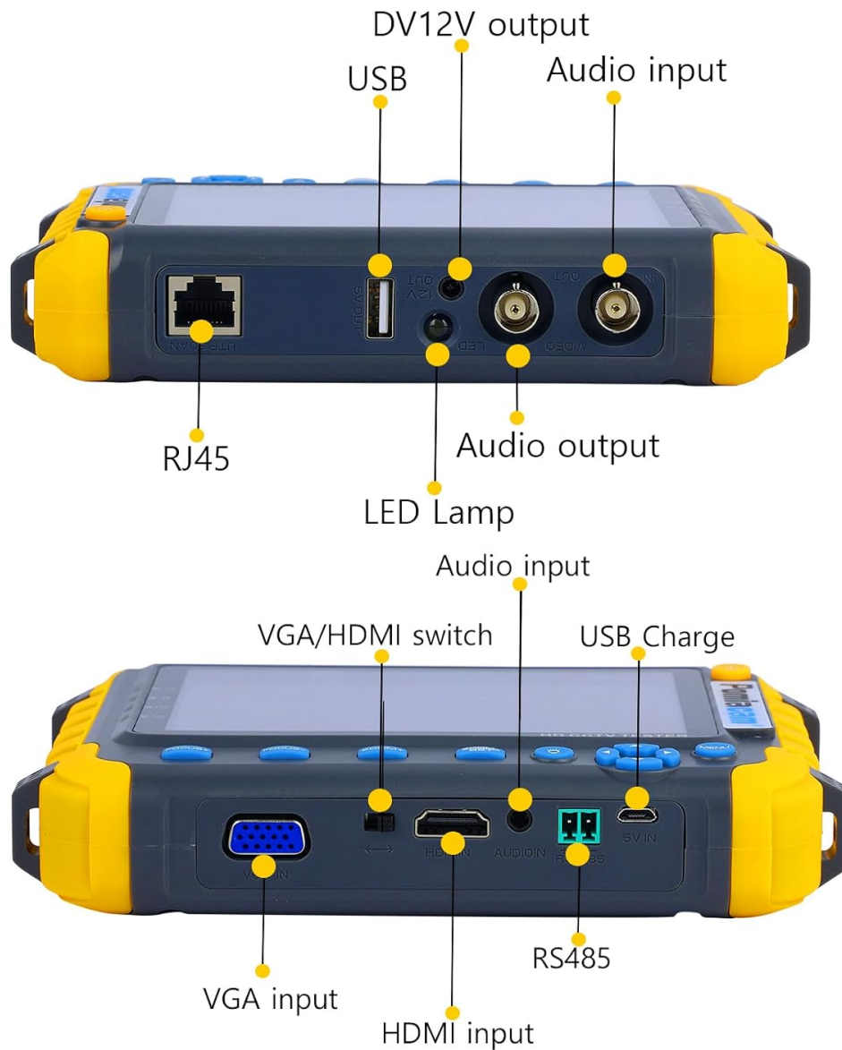
Image: Top and bottom views of the POMIACAM IV8W tester, highlighting ports such as RJ45, USB, DC12V output, Audio input/output, VGA input, HDMI input, and RS485 terminals.
