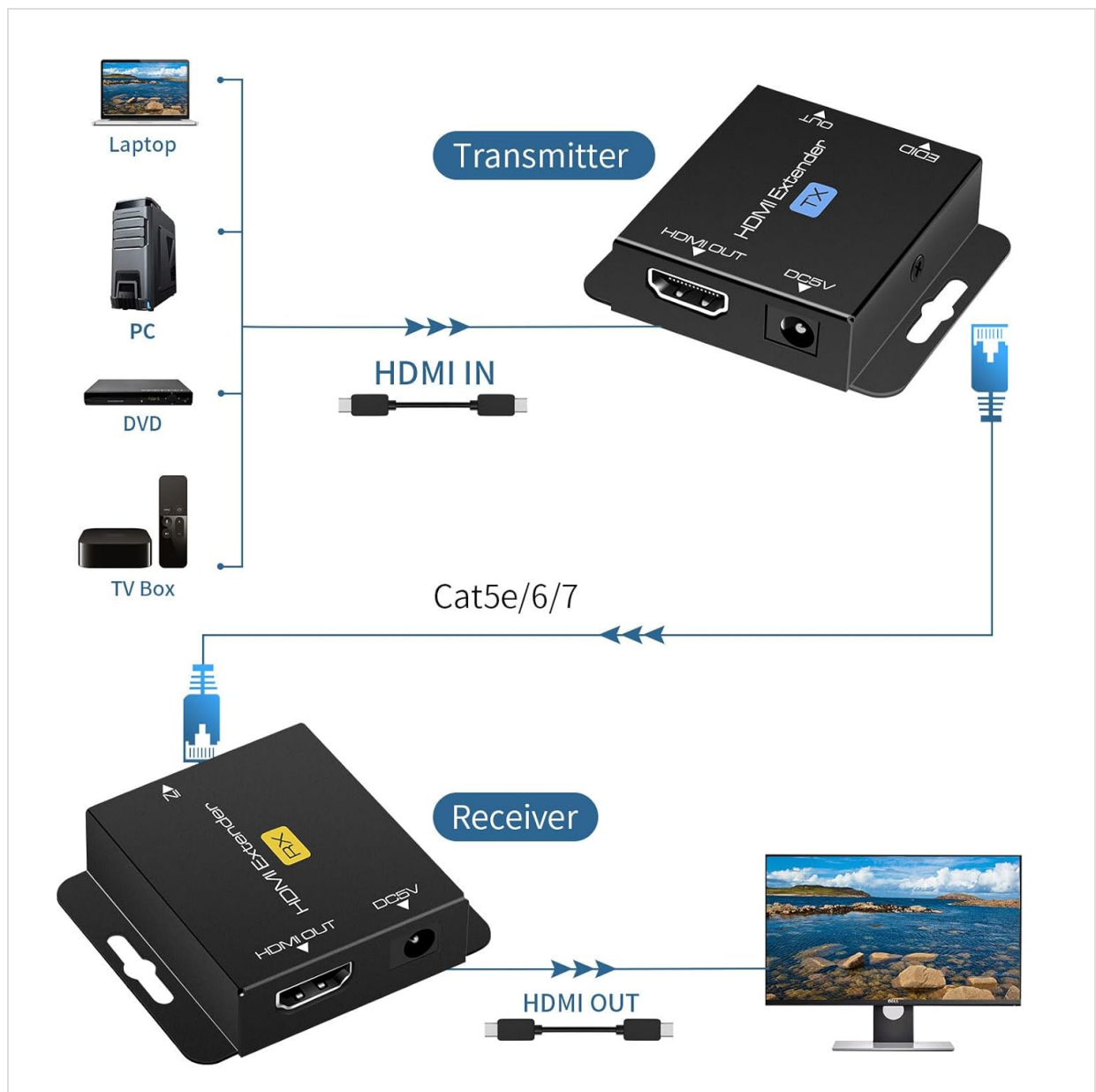
Image: Diagram illustrating how to connect the HDMI extender: a source device (laptop, PC, DVD, TV Box) connects to the TX unit via HDMI, the TX unit connects to the RX unit via a Cat5e/6/7 cable, and the RX unit connects to a display via HDMI.
