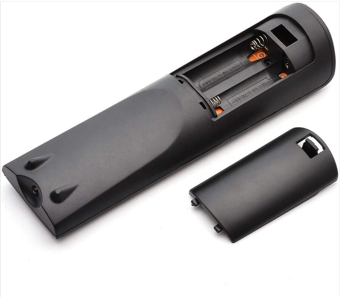
Figure 1: Battery compartment with cover removed, illustrating correct battery placement.
