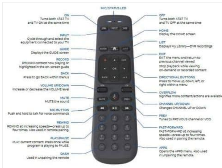
Figure 2: Detailed diagram of the remote control with button functions.
