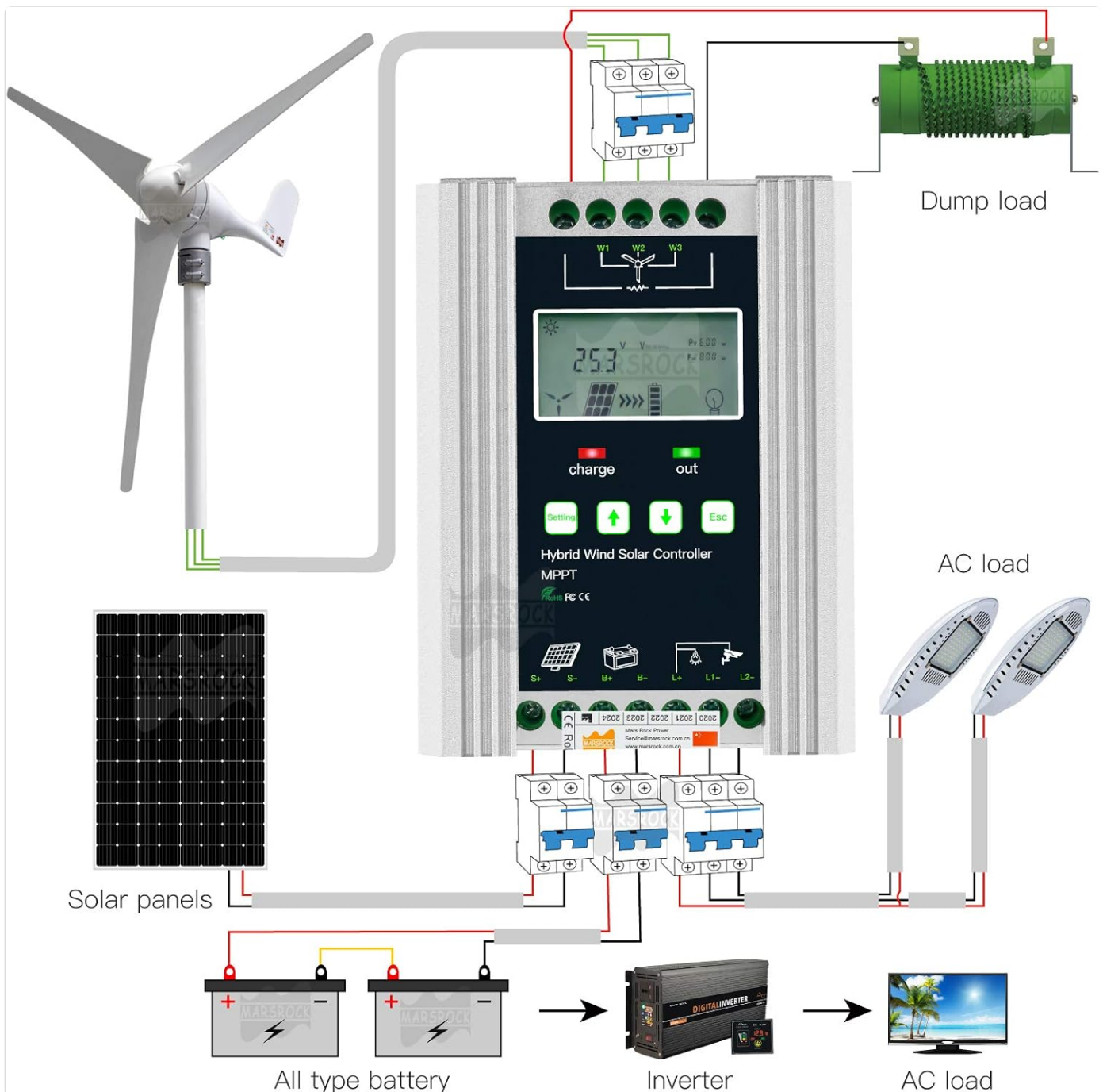
Image 5.1: Comprehensive wiring diagram for the hybrid system.
