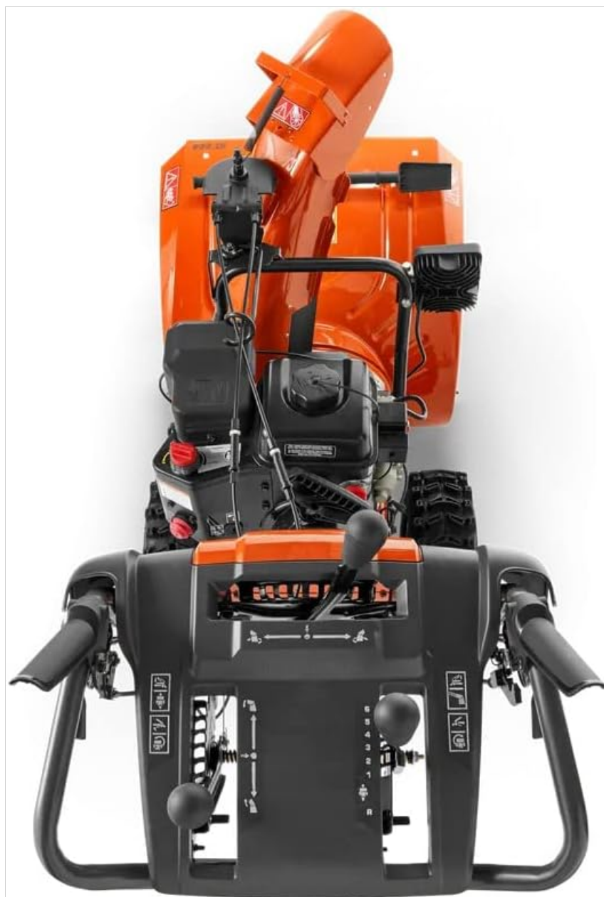
Image: A top-down view of the snow blower's control panel, showing levers for drive, auger, and chute control.
